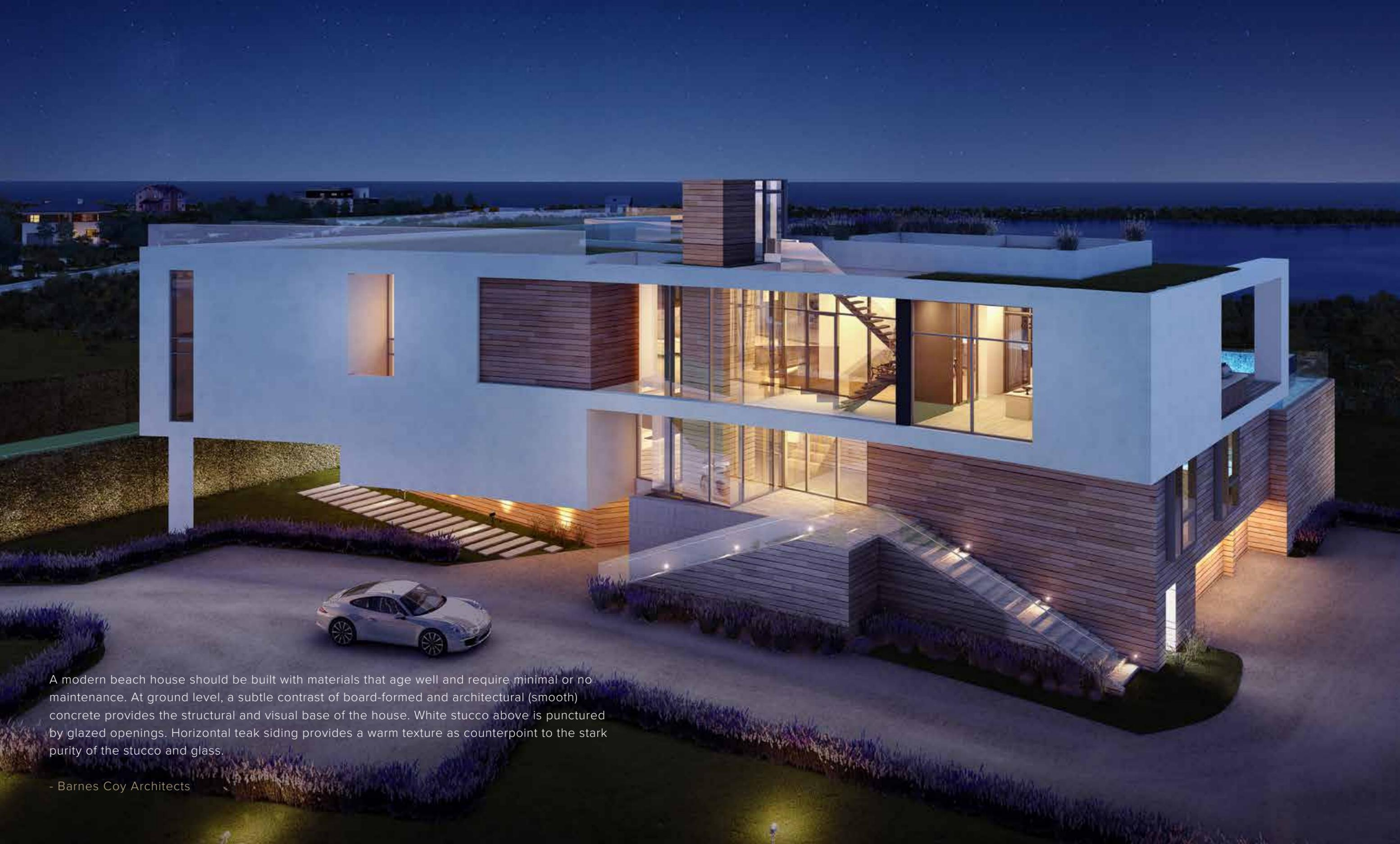
A modern beach house should be built with materials that age well and require minimal or no maintenance. At ground level, a subtle contrast of board-formed and architectural (smooth) concrete provides the structural and visual base of the house. White stucco above is punctured by glazed openings. Horizontal teak siding provides a warm texture as counterpoint to the stark purity of the stucco and glass.
